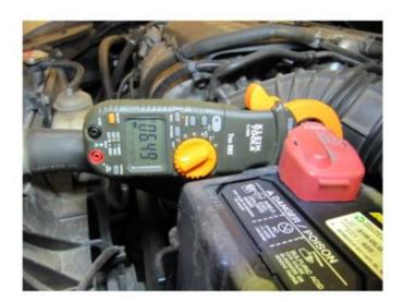
Now, turning on the blower Fan to HIGH:  $\sim$ 21Amps load, ELD =  $\sim$ 3.24V
