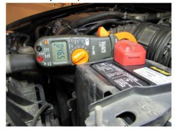
Also turning on the AC (so the radiator fans come on):  $\sim$ 57.5Amps load, ELD =  $\sim$ 1.2V
