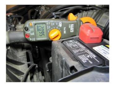
Additionally turning on the Rear Defroster:  $\sim$ 36Amps load, ELD =  $\sim$ 2.4V
