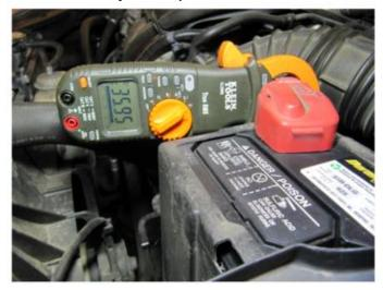
Additionally turning on the headlights:  $\sim$ 46.5Amps load, ELD =  $\sim$ 1.8V
