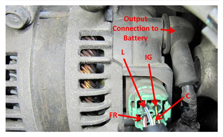
**IG** = Keyed battery power supplied to the voltage regulator. Should be equal to battery voltage when Key is in the ON position and when engine is running.
