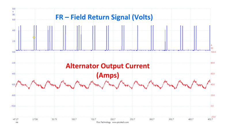
The average alternator current is now 39.5Amps and the FR signal is high only 4.5% of the time, so it is low 95.5% of the time, indicating that the alternator is working at 95.5% of its full capacity.
