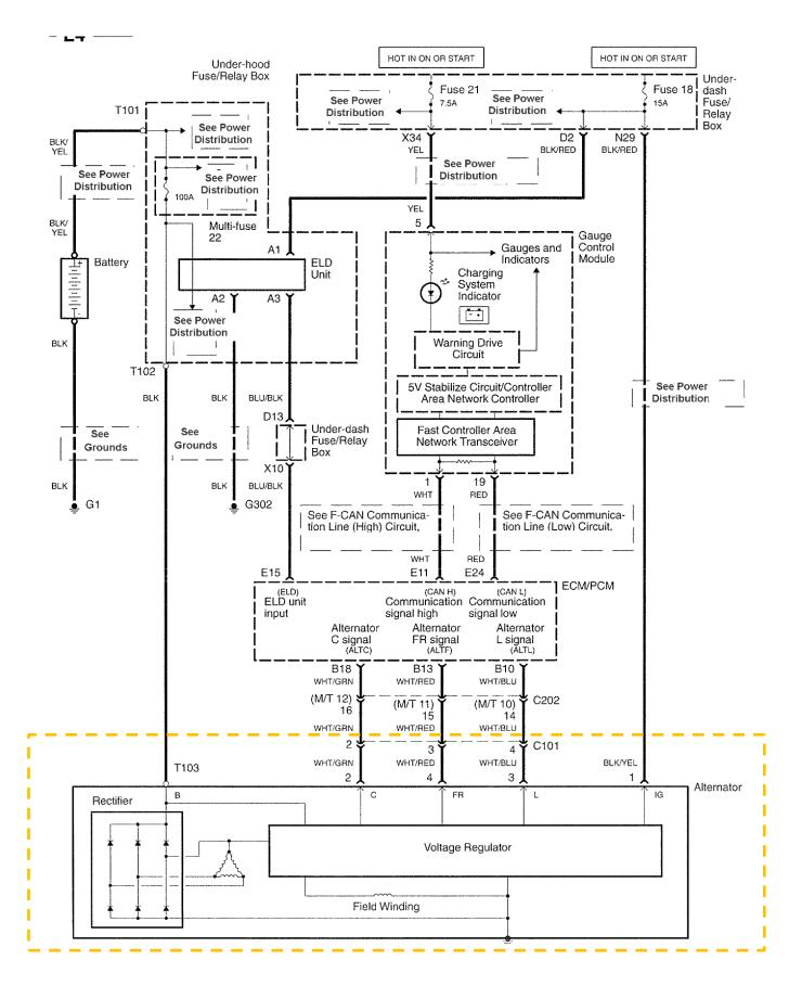
2007 4CYL Accord 2.4L Alternator Signals and Known-Good Waveforms
