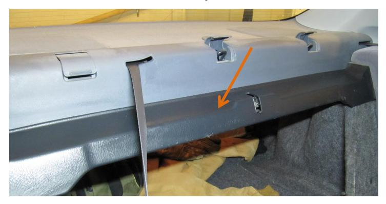
This trim piece has white clips that hold it in place from the top, and then on the bottom it hooks around the metal frame of the top of the trunk opening. I think you are supposed to remove the side seat sections to gain better access, but I wrestled it out by unhooking the front edge and then prying it up in the rear on the top:
