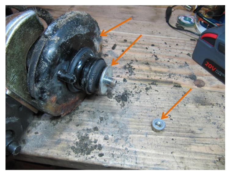
Remove the lock nut, the top washer, and the top plate:
