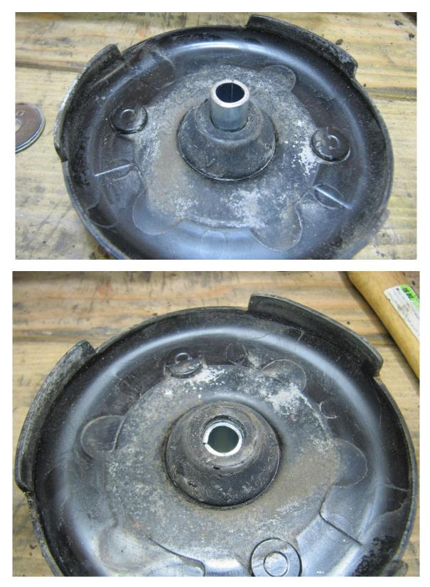
Install the collar and push into the two rubber bushings (I used a new collar for reassembly):
