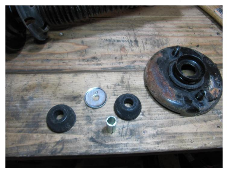
I used new rubber mounts, a new collar, and a new washer for reassembly:
