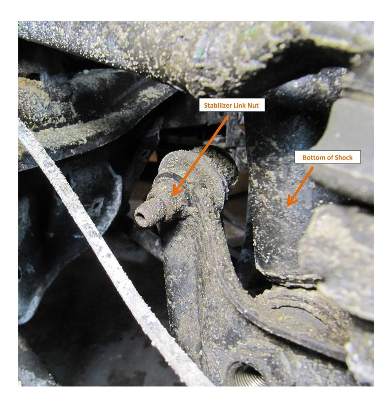
The stabilizer link nut can be notoriously difficult to get off because the bolt tends to just spin in the stabilizer joint. I figured I was probably going to have to just cut it off and replace the link, but I actually did succeed in getting the nut off on both sides. I found that it helped to clean up the threads first. I used a dremel and wire wheel, but a small wire brush probably would have worked as well.
