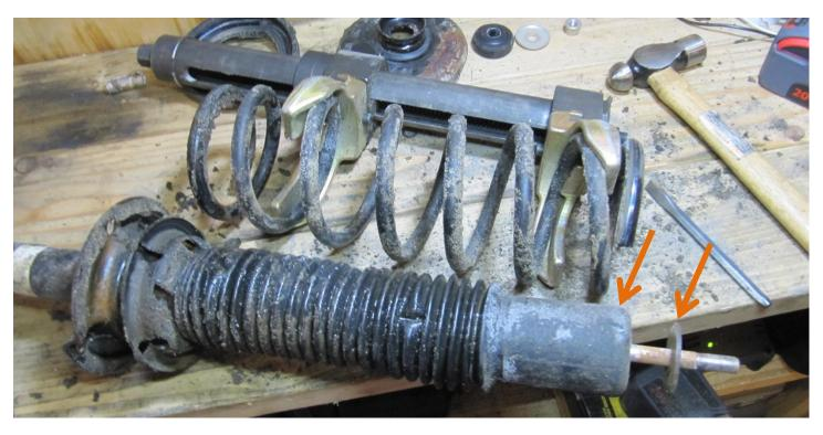
Next, slide off the dust cover cap (basically a washer) and the dust cover.
