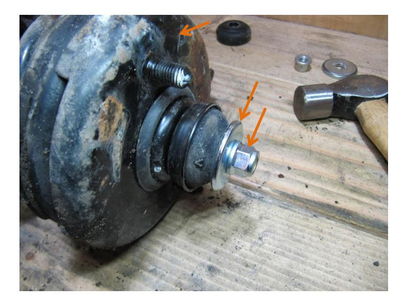
Install the top plate, the washer, and a new locking nut:
