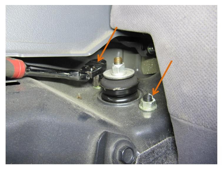
The service manual recommends removing the top of the stabilizer link so that there is sufficient room to remove the strut and get it out. It may be possible to avoid removing the stabilizer link, but I am not sure – it is pretty tight.
