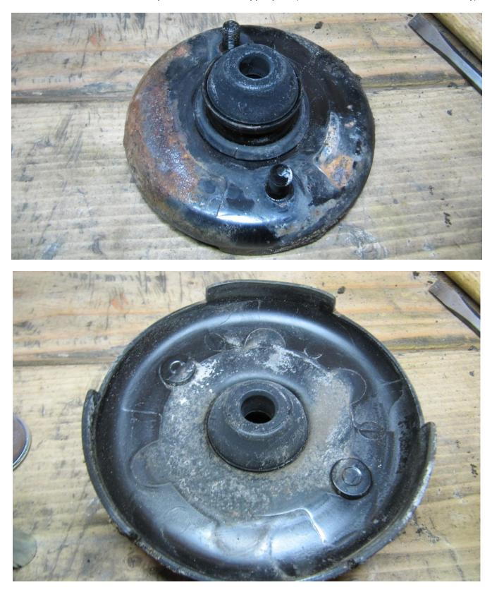
Insert the rubber mounts in the top and bottom of the upper plate (I used new rubber mounts for reassembly):
