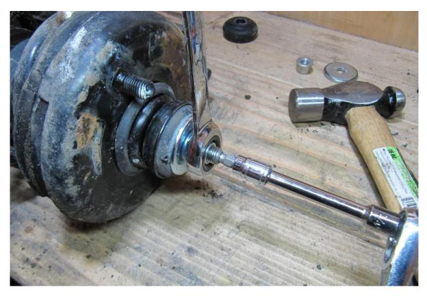
Use a 5mm Hex Socket in the shock end to keep the shock from turning as you tighten the lock nut:
