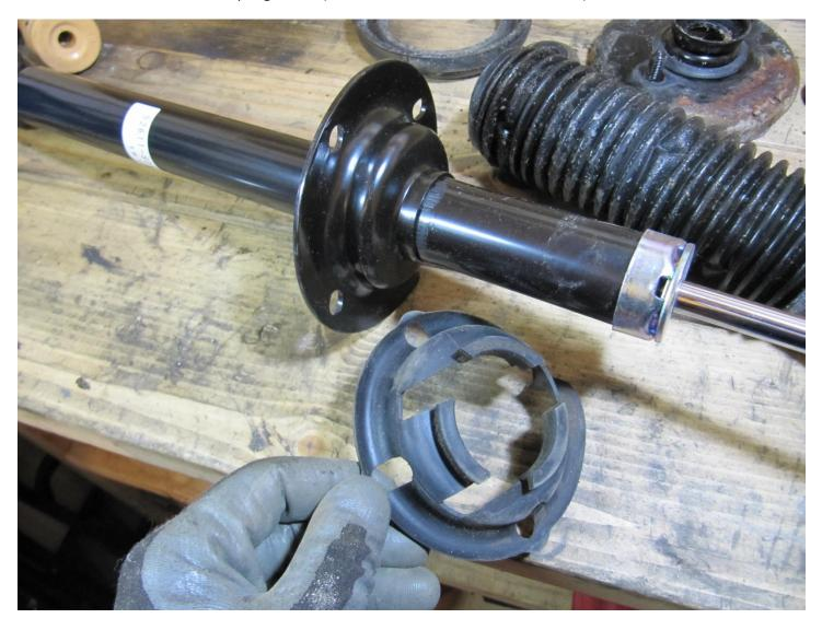
Now, you'll need to clean off and reassemble the parts onto the new shock absorber, starting with the rubber bottom spring mount (which is also the base of the dust cover):
