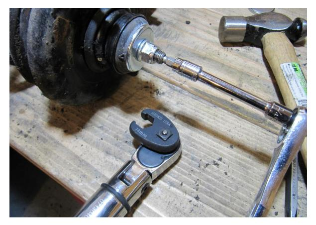
Line up the spring so that the bottom spring end lines up with the pocket. Also, line up the top cap so that a straight line through the two bolts lines up with the direction of the bushing on the bottom of the shock. When everything is lined up as it should be, release the tension on the spring.
