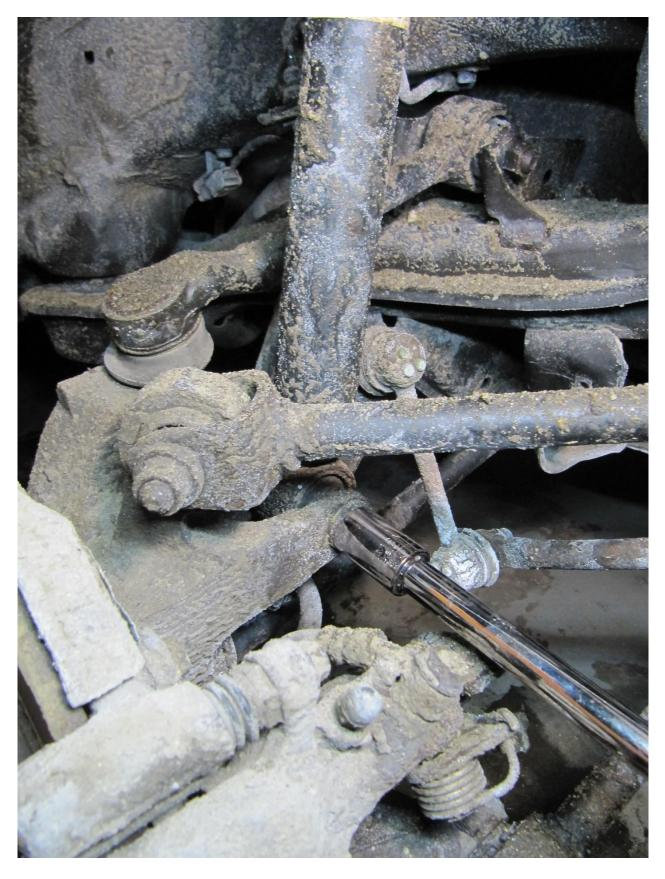
Remove the bolt holding the strut to the knuckle:
