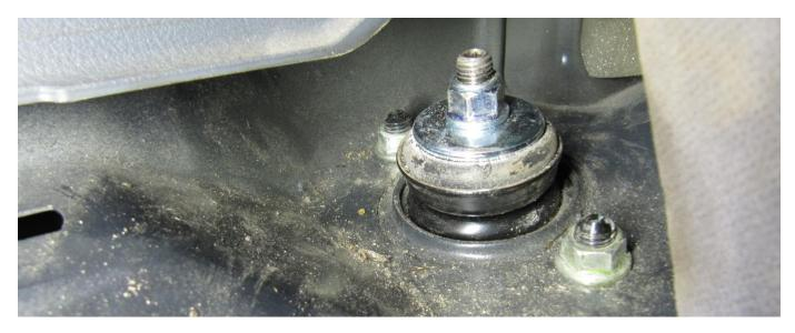
Put the strut into position and reinstall the two nuts to hold the top of the strut in place:
