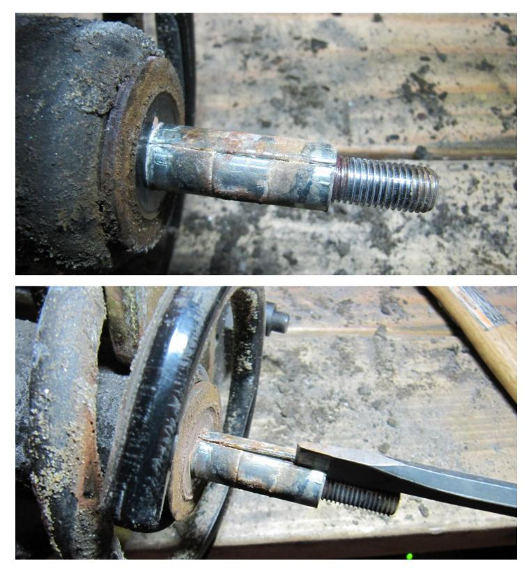
Next, you will need to remove the split-collar. Mine was quite stuck and I used a cold chisel to split it open and remove it:
