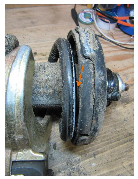
Compress the spring until there is play between the spring and the top and bottom plates (the spring should wiggle freely from the shock):
