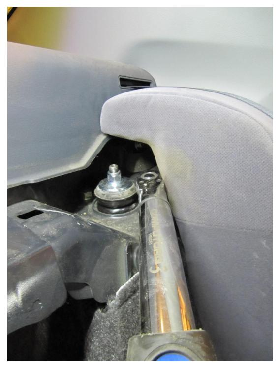
Finally, torque the top mounting nuts to 50 N-m:
