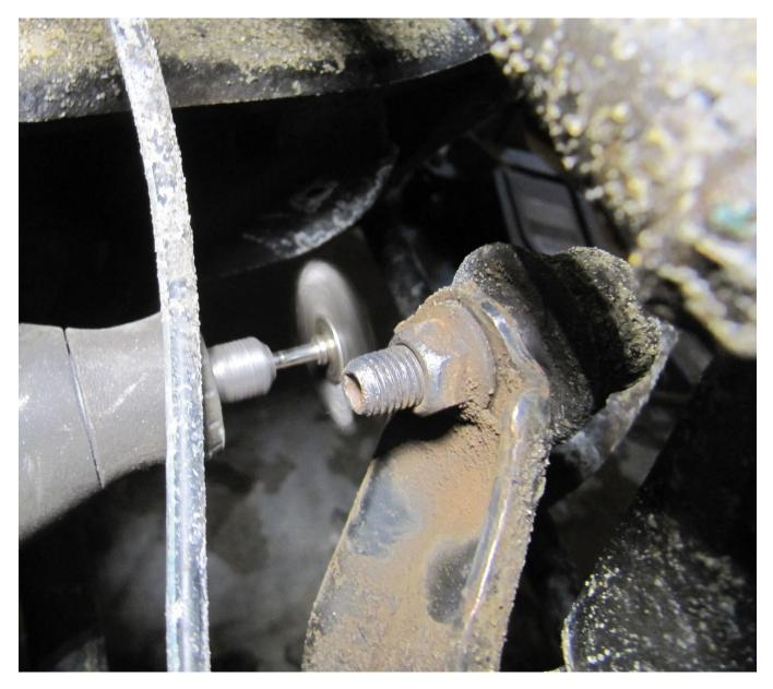
First, I broke the nut free with a socket and ratchet. Then I used a 5mm hex socket to keep the bolt from turning. But you probably can't put a whole lot of torque on it before it will strip out (which is why cleaning up the threads helped a lot in getting the nut off).
