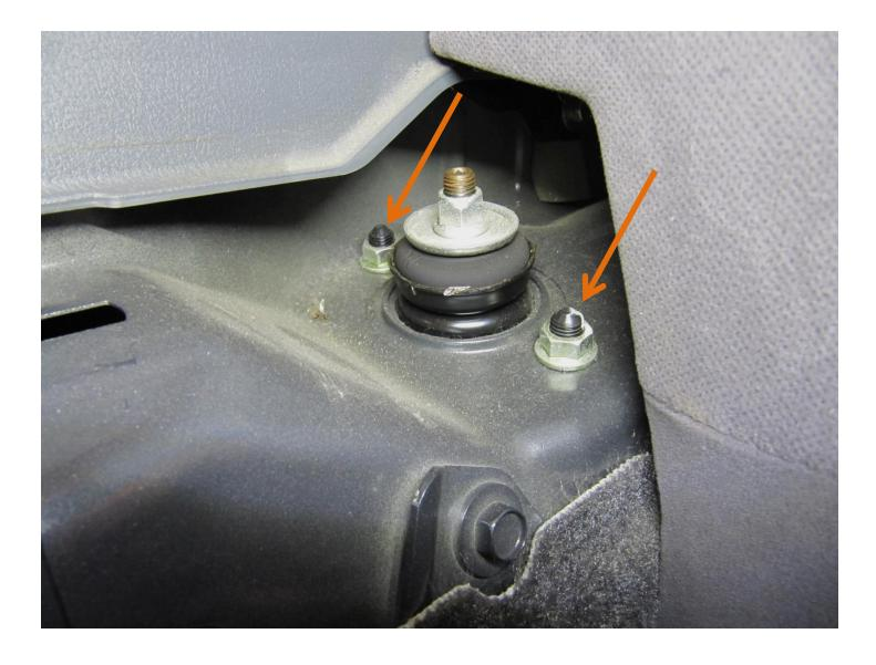
This provides access to the two nuts holding the rear strut in place as shown below:
