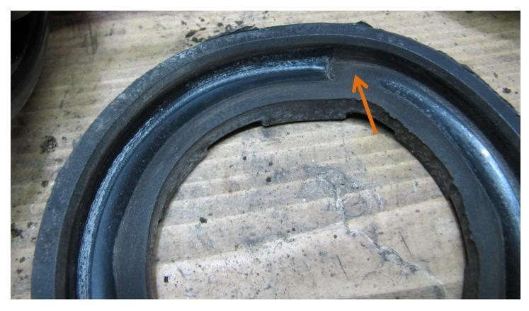
On the top rubber mount, you can see where the end of the spring rested previously.
