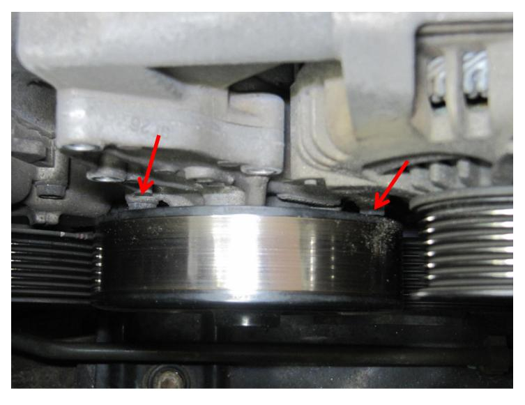
There are two bolts behind the water pump pulley:
