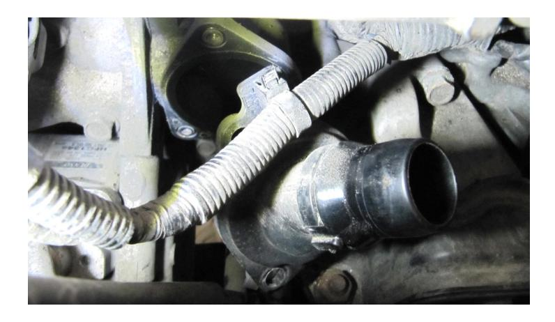
Once the bolts are removed, pull out the old thermostat:
