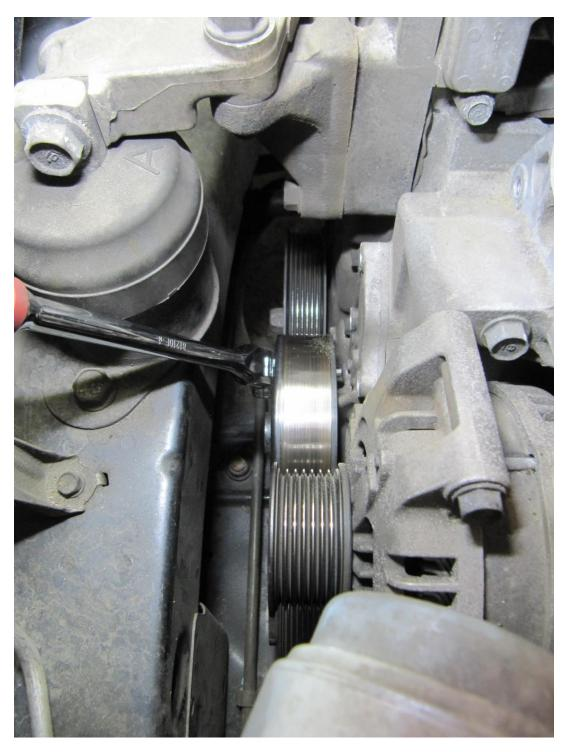
These bolts can be accessed through the holes in the water pump pulley as shown:
