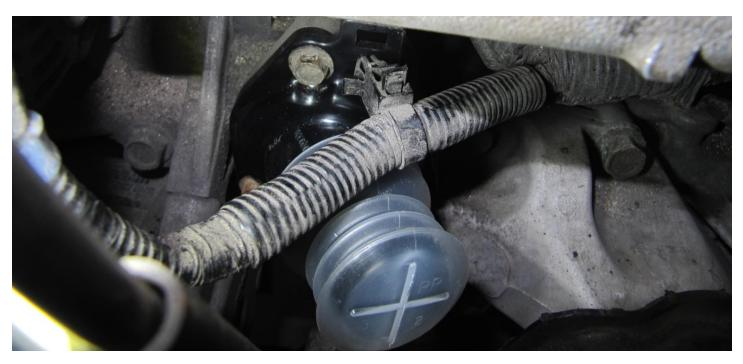
Install the new thermostat and torque to 9.8 N-m:
