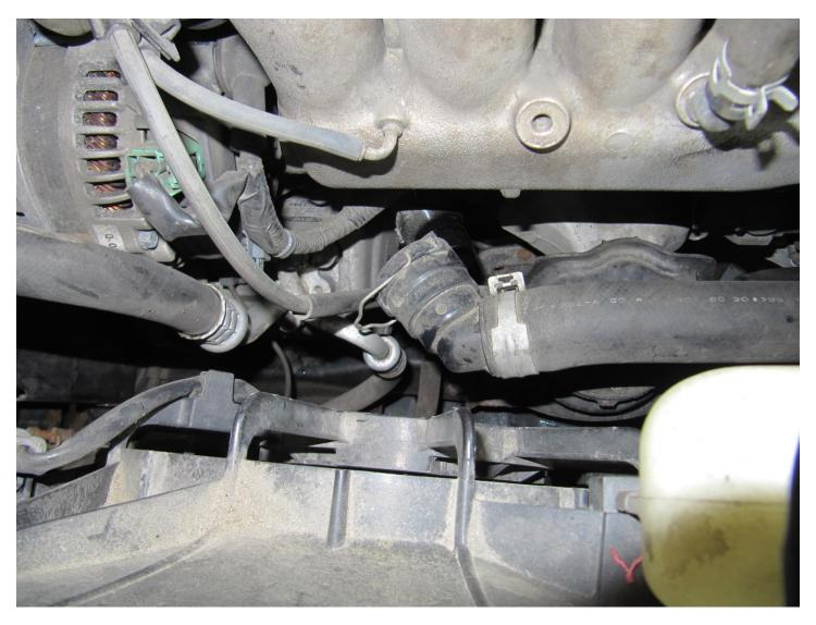
Then pull the hose and quick-connect off the thermostat:
