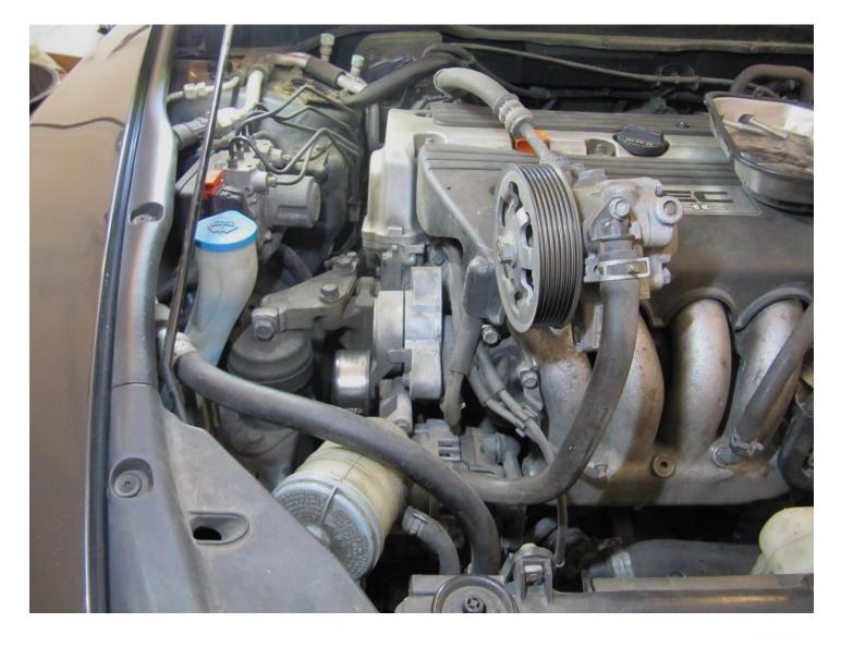
Leave the hoses connected and pull the power steering pump off to the side (it helps to unhook the power steering reservoir)
