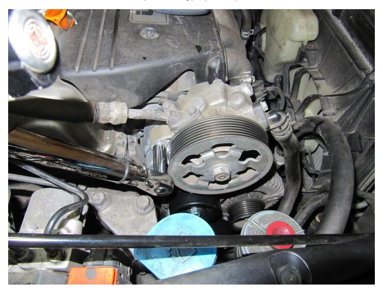
Reinstall the power steering pump and torque to 22 N-m:
