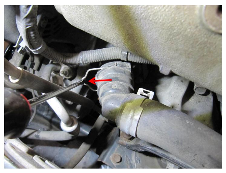
To replace the thermostat, pull the quick-connect tab to the left:
