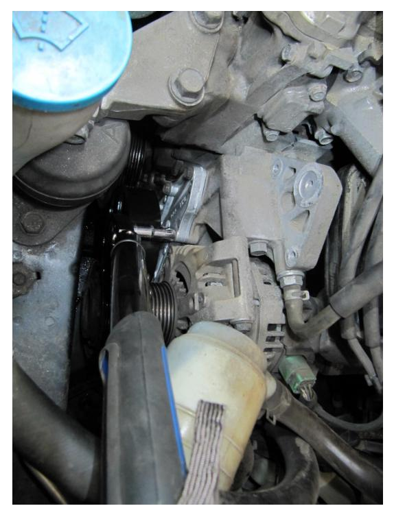
Re-insert the bolts and tighten to 12 N-m:
