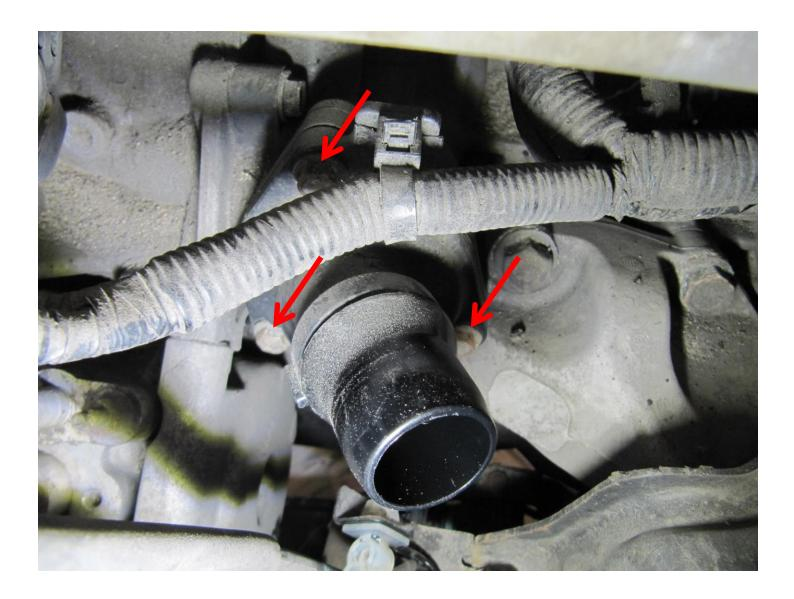
To provide a little more working room, it helps to remove the alternator wire tie from the back of the alternator (pinch ears and the tab can be removed). This allows the wire to move freely providing more room to access the thermostat bolts behind it:
