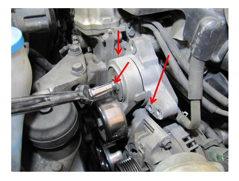
Remove the three bolts holding the belt tensioner. Notice that there is one bolt in the center where the tensioner rotates:
