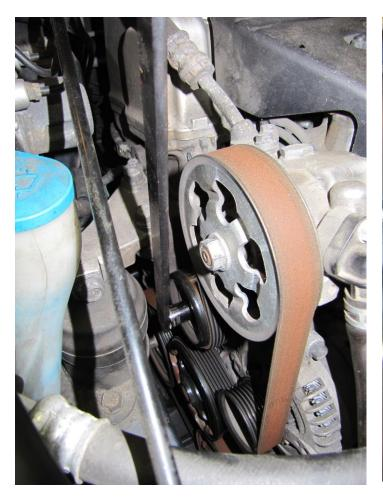
Rotate the tensioner to relieve the belt tension and remove the serpentine belt:
