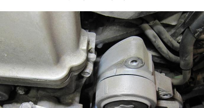
The bolt on the far side of the tensioner is a bit of a pain to get too (it is a tight fit around the engine mount) but you can get it with the right length socket:
