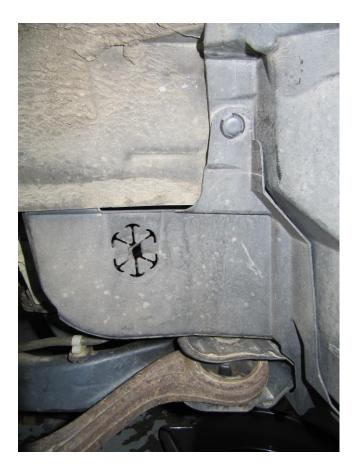
It might be easiest to get to the bottom bolt on the water pump from the underside. Remove the two clips holding the panel behind the passenger side wheel:
