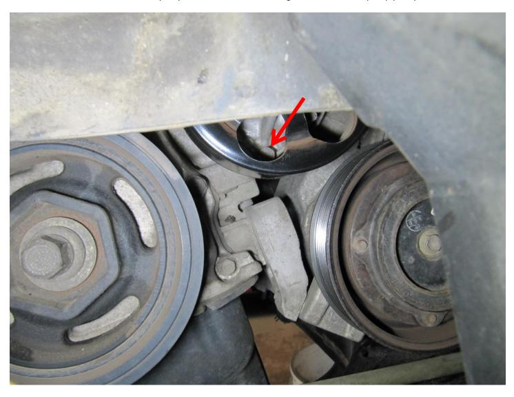
The final water pump bolt is shown here, hiding behind the water pump pulley:
