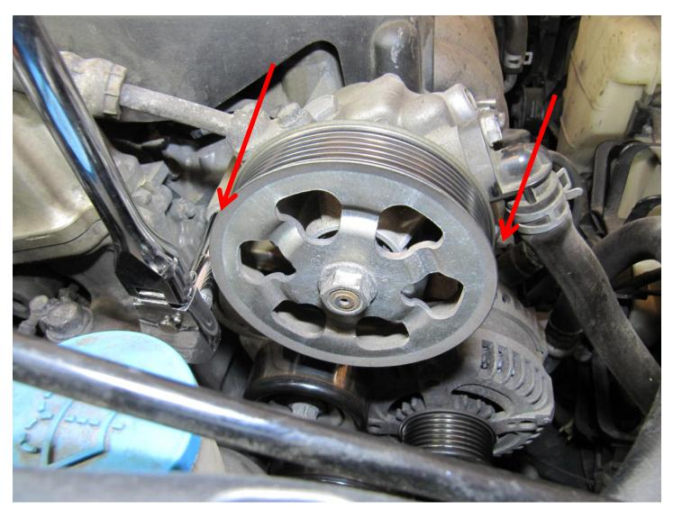
Remove the two bolts holding the power steering pump (but leave the hoses connected):
