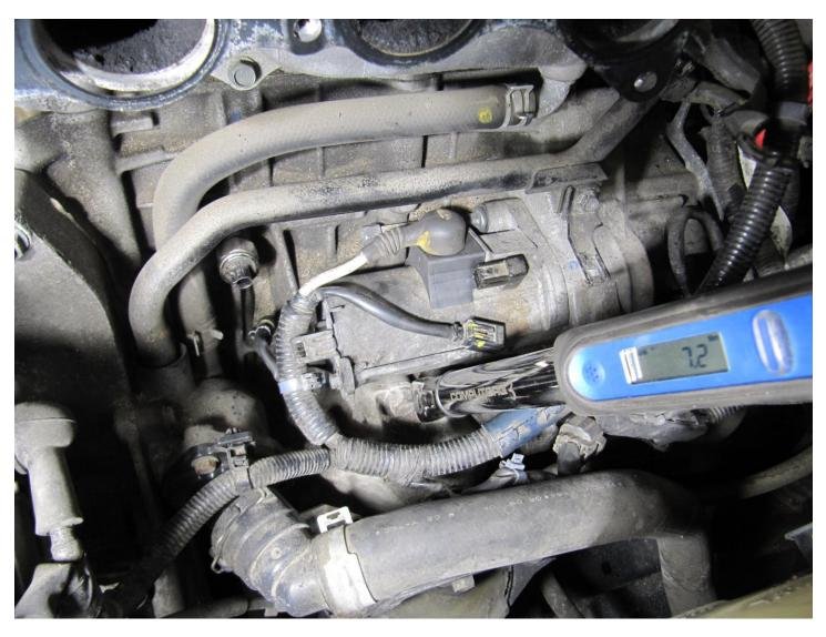
The front bolt gets torqued to 64 N-m. The rear gets torqued to 44 N-m.
