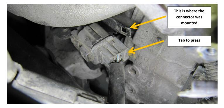
Looking up under the intake manifold, there is another connector on that same cable but it is really difficult to get access to. I left it connected for now and disconnected it later when the intake manifold was loose allowing better access:
