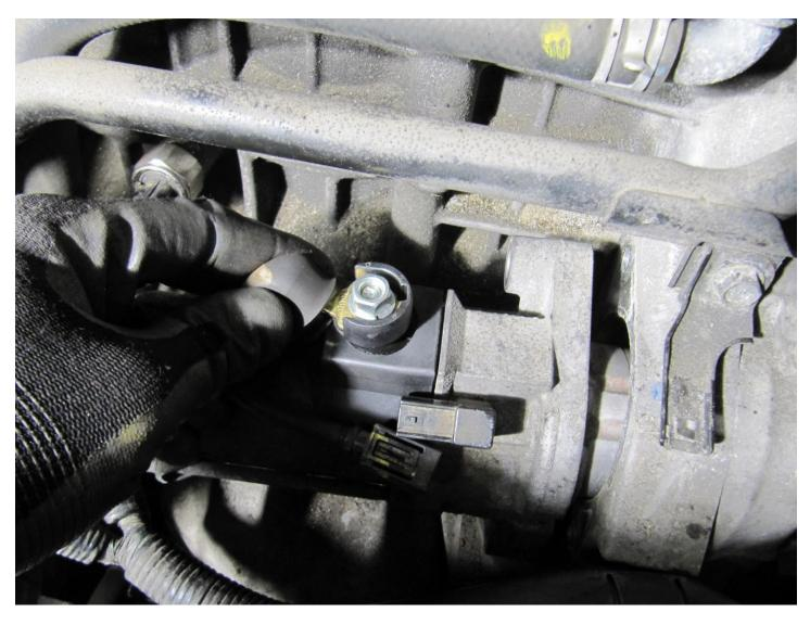
Reassembly! Make sure you put on the electrical connector before putting the starter fully into place:
