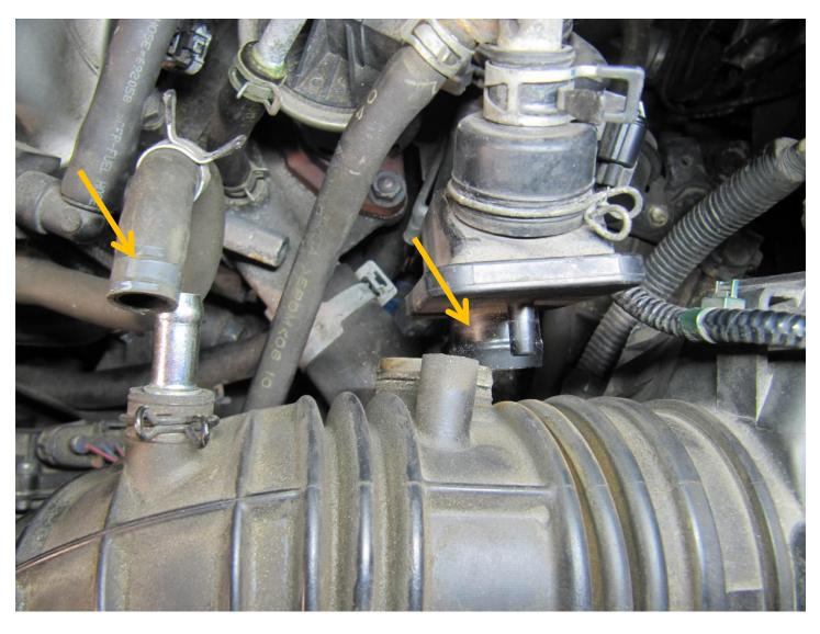
Remove the vacuum hose and breather pipe from the intake air duct:
