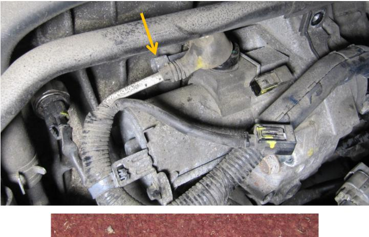
And remove the rear starter bolt, which is an extension bolt to make it easier to reach:
