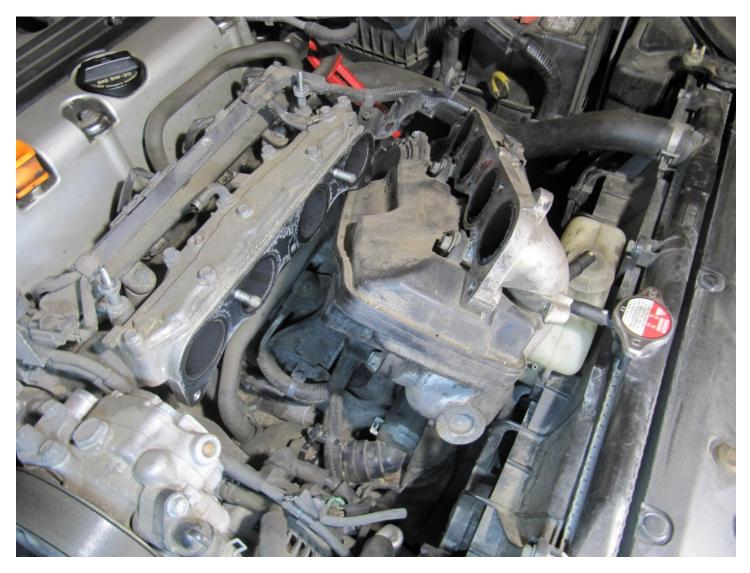
Now the intake manifold is largely free, but REMEMBER the wire harness is still connected on the bottom so GENTLY shift it off to the side as shown below:
