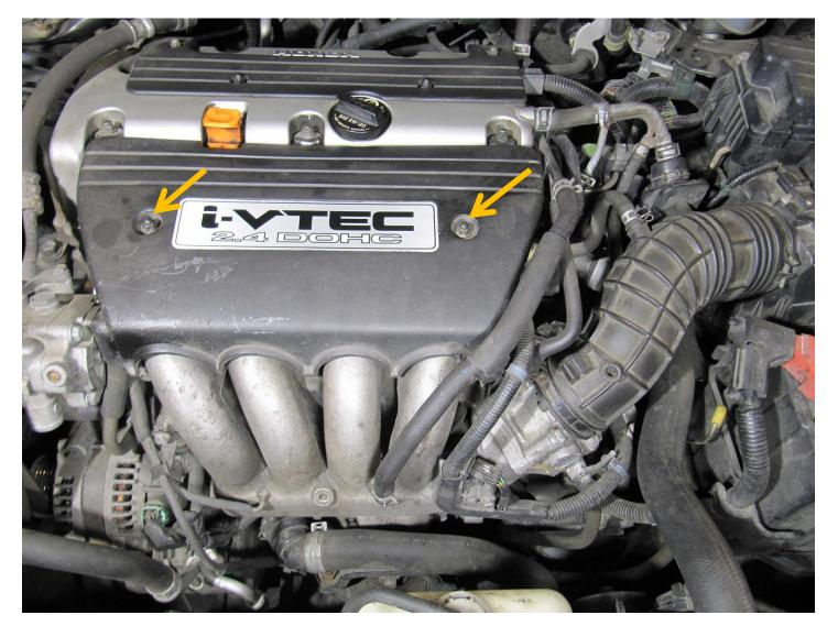
Remove the two nuts and the engine cover:
