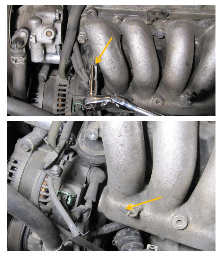
Remove the vacuum line bracket and the vacuum hose:
