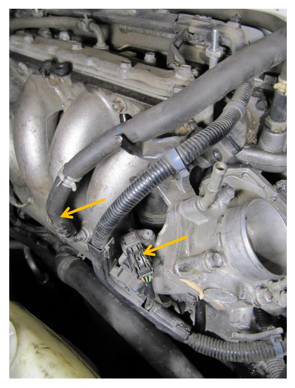
Reinstall the brake booster vacuum line and MAP electrical connector:
