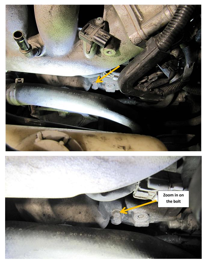
This step is probably not obvious, but there is a bracket attached to the bottom of the intake manifold that needs to be disconnected from the engine. You will need to reach down and remove the bolt shown below:
