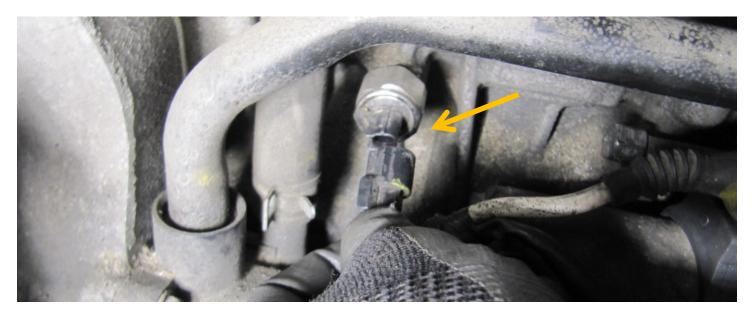
Reconnect the cable clamps and electrical connector:
