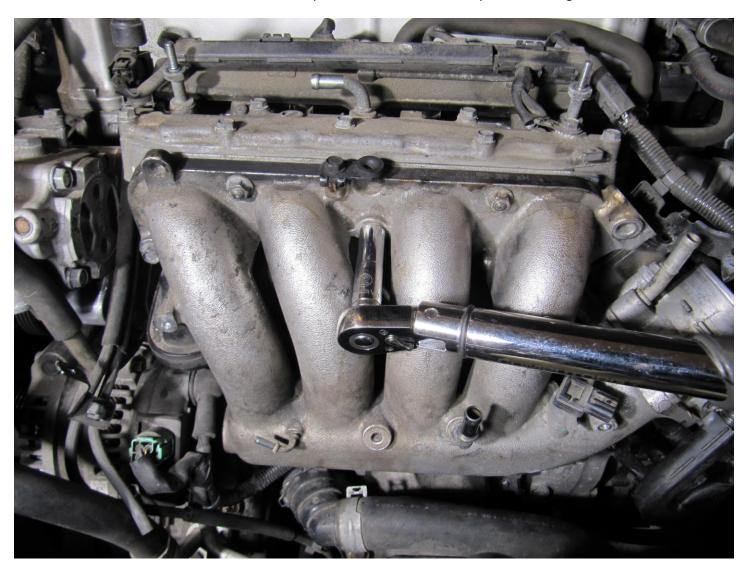
Reinstall the intake manifold and torque to 22N-m in a crisscross pattern starting at the center:
