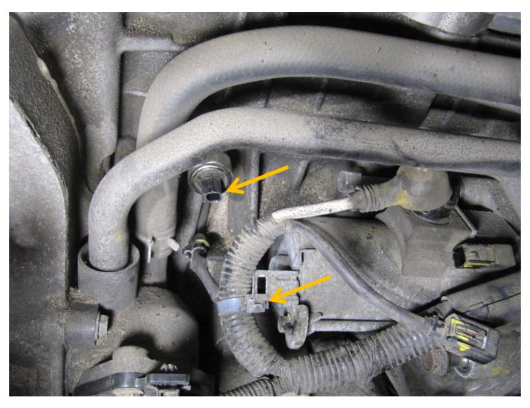
Remove the knock sensor connector (to give yourself more room to access the rear bolt) and the wire harness clip:
