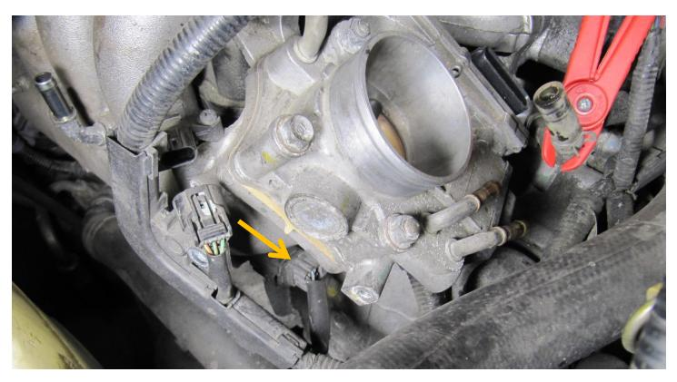
Remove the electrical connector below the throttle body:
