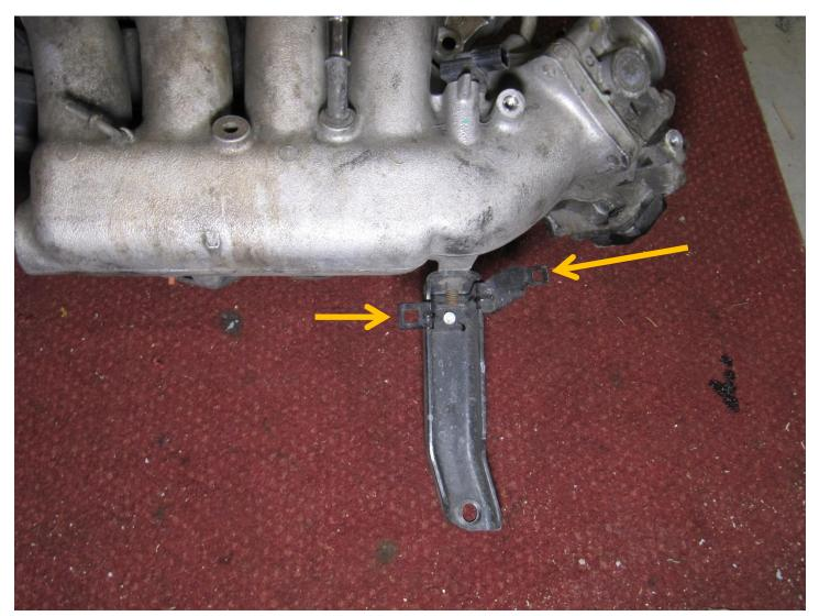
Now that the intake manifold is removed, you can see the lower bracket as well as the locations where the electrical connector was fastened (arrows):
