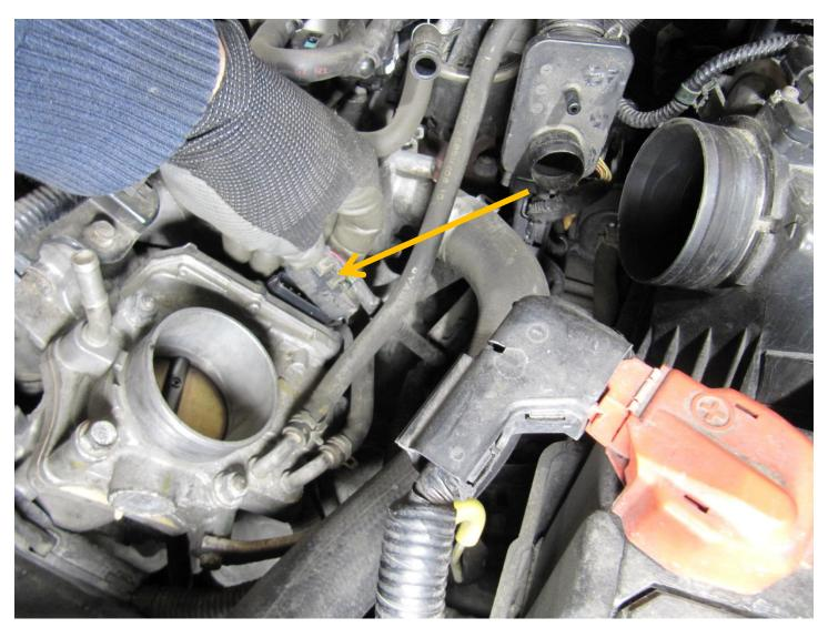
Remove the throttle body electrical connector:
