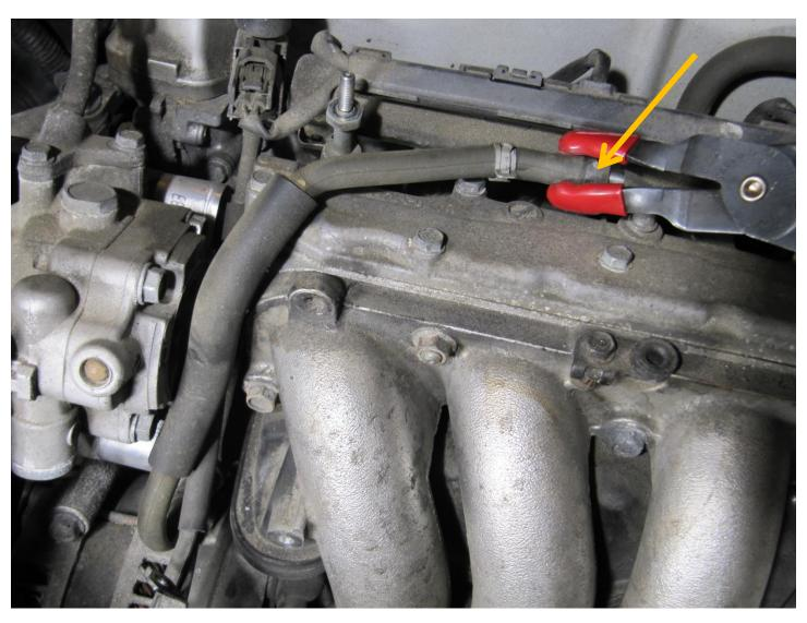
You could probably leave the PCV valve hose connected, but I removed it just to provide a little more working room:
