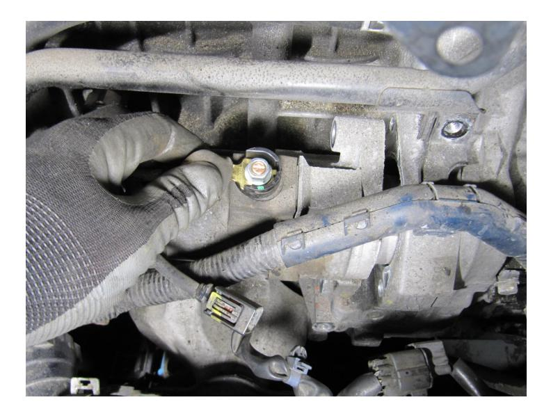
Now, the starter can be shifted outward to gain access to the electrical terminal:
