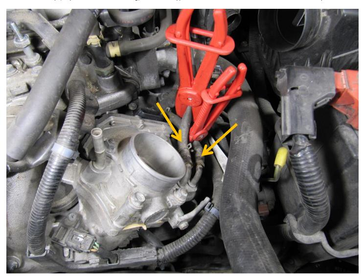
Clamp (to prevent coolant leaking) the water bypass hoses and disconnect from the throttle body:
