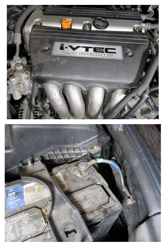
And obviously, reinstall the engine cover and negative battery terminal:
