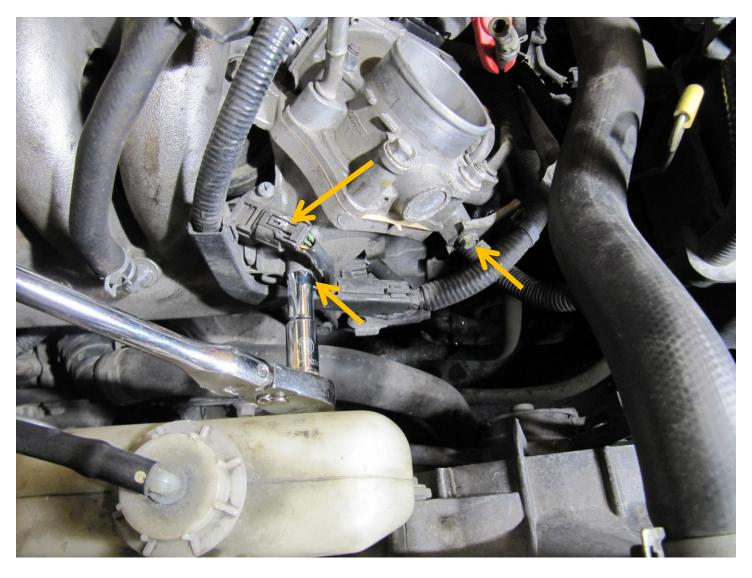
Disconnect the MAP sensor electrical connector and the two bolts holding the electrical cable:
