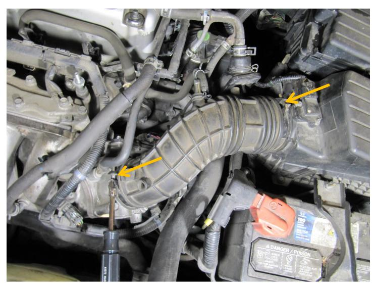
Reinstall the intake air duct and tighten the band connectors on both ends (5.5mm socket I believe):
