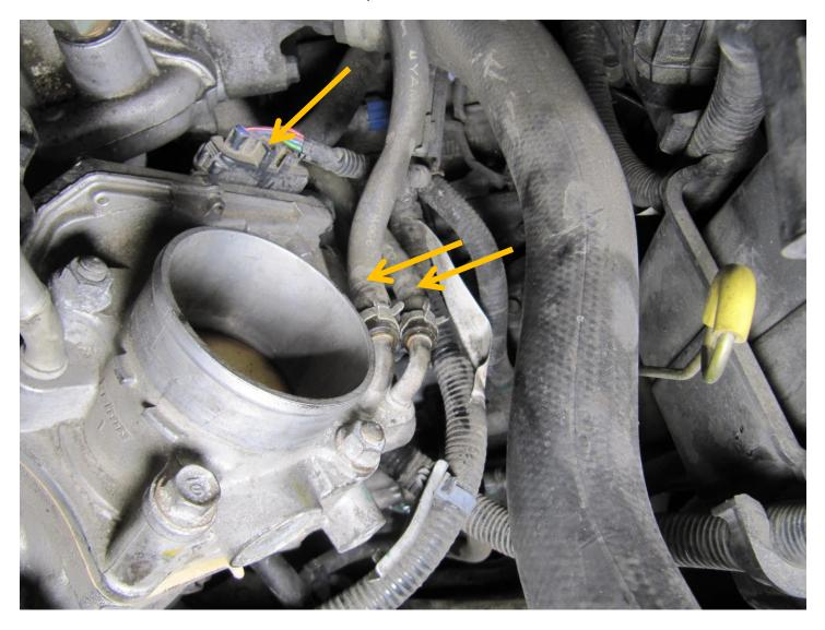
Reinstall the throttle body electrical connector and coolant lines:
