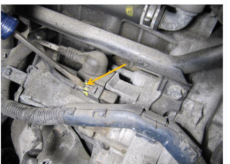
Depress the tab to remove the small electrical connector (I believe this provides power to the solenoid, which in this starter is integrated into the starter itself):
