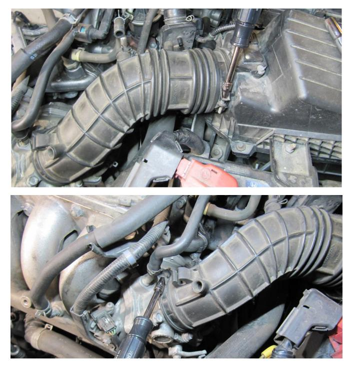
Loosen the clamps on both ends of the intake air duct:
