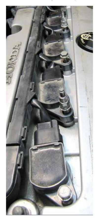
Finally, replace the ignition coil cover and install its bolts.
