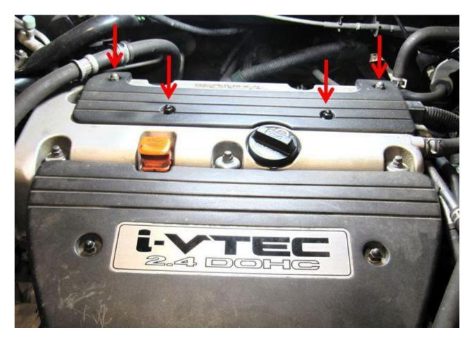
Remove the four bolts holding in the ignition coils:
