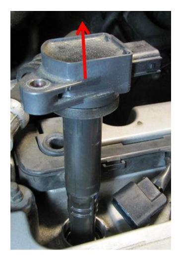
Inspect ignition coils. Any oil on the ignition coil indicates a failing spark plug tube seal in the cylinder head cover.
