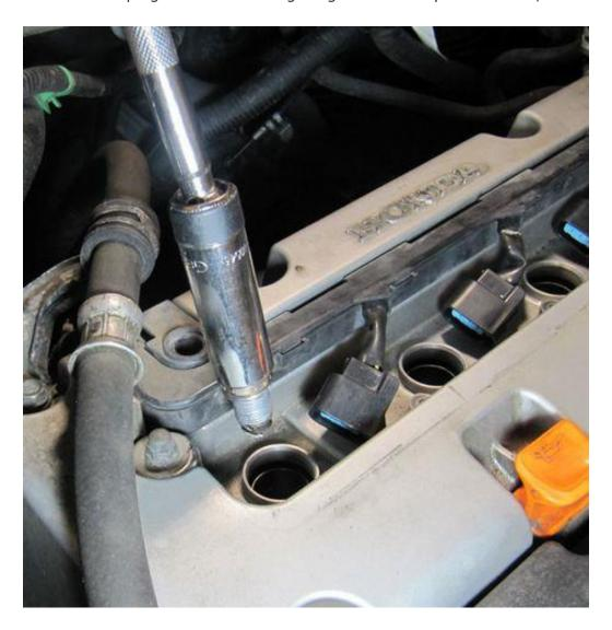
Re-install ignition coils and their electrical connectors. Insert ignition coil bolts with the longer ones in the locations shown. Torque to 12N-m, 8.7ft-lb.
