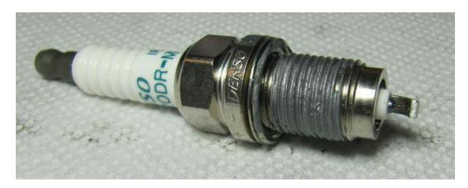
Insert the new plug and screw in finger tight. Then torque to 18N-m, 13ft-lb.
