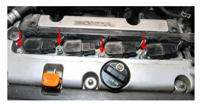
Remove the electrical connector from each ignition coil:
