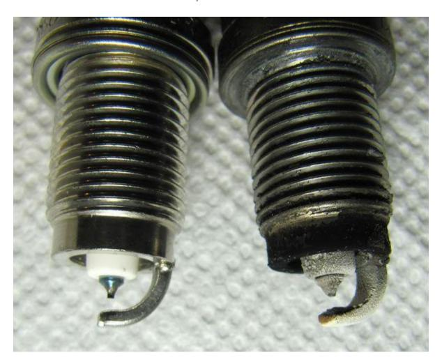
Per the Honda Service Manual, apply a small amount of anti-seize to the new plug threads.
