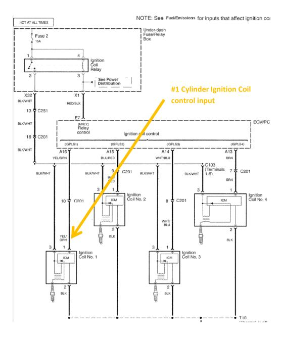
Back-probes can be used to probe the ignition control input to the #1 cylinder ignition coil via the back of the connector as shown below. The scope probe is hooked to the control wire (green/yellow) and the scope ground is hooked to the ground wire (solid black). Notice that cylinder #1 is closest to the crank pulley (Serpentine belt) and the cylinders are number 1,2,3,4 across with 4 being on the transmission side of the engine.
