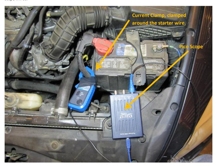
With the current clamped around the starter motor wire as shown above, the engine was cranked over to produce the following waveform (I also disconnected all the fuel injector connectors to avoid flooding the engine). The peak of each bump represents the point of maximum compression in an individual cylinder. In this case, there are no major compression differences between cylinders since all of the bumps have about the same amplitude (height).
