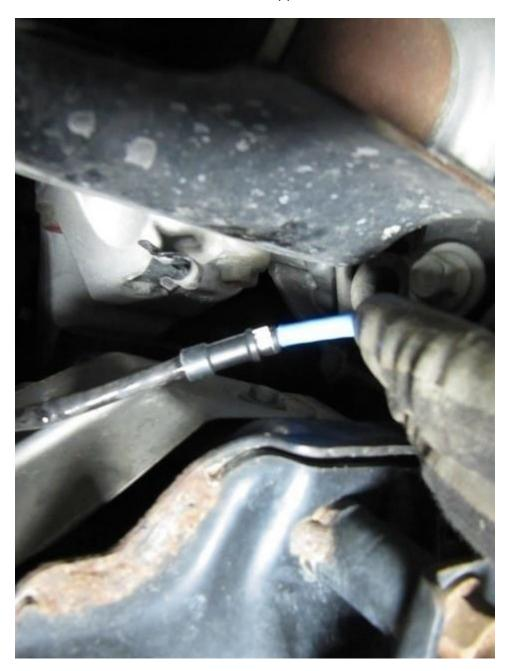
When installing the new oxygen sensor (I replaced with an OEM replacement unit) the torque is 33 ft-lb:
