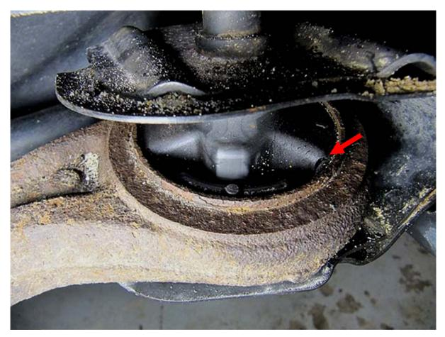
There are three Lower Control Arm Bushings: Compliance Bushing, Shock Absorber Bushing and Rear Bushing. Per the Honda service manual, the following bolts and nuts should be replaced with new parts when re-installing the lower arm (per the service manual): 20, 21, 19, 18, 16.
