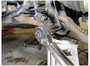
Torque the Lower Ball Joint nut to 58 ft-lbs.
