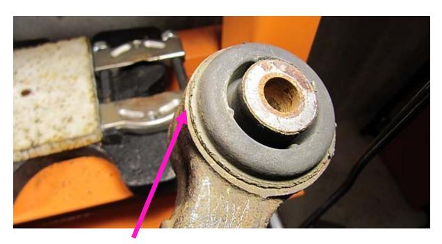
The metal collar leaves very little of the control arm exposed to support when pushing out the bushing
