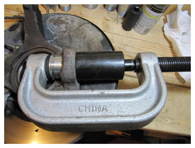
Here is the ball joint once it is fully pressed in and a picture of the newly installed ball joint:
