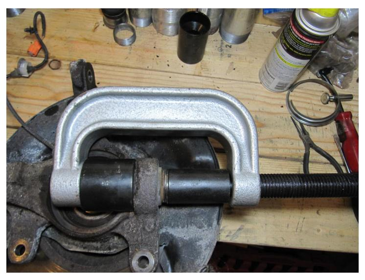
I use a C-Frame Press with the OTC 6734 adapters to press out the old ball joint.
