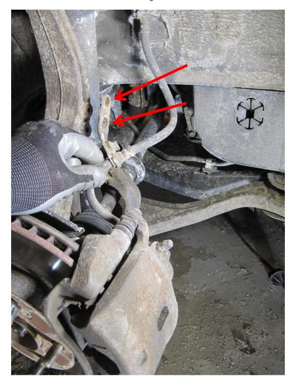
Remove the two bolts holding the caliper bracket (and entire caliper) onto the knuckle:
