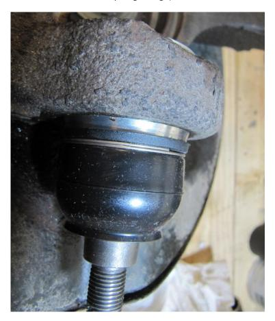
Reinstall the dust ring, lining up the gap in the ring with the ABS sensor (arrow):
