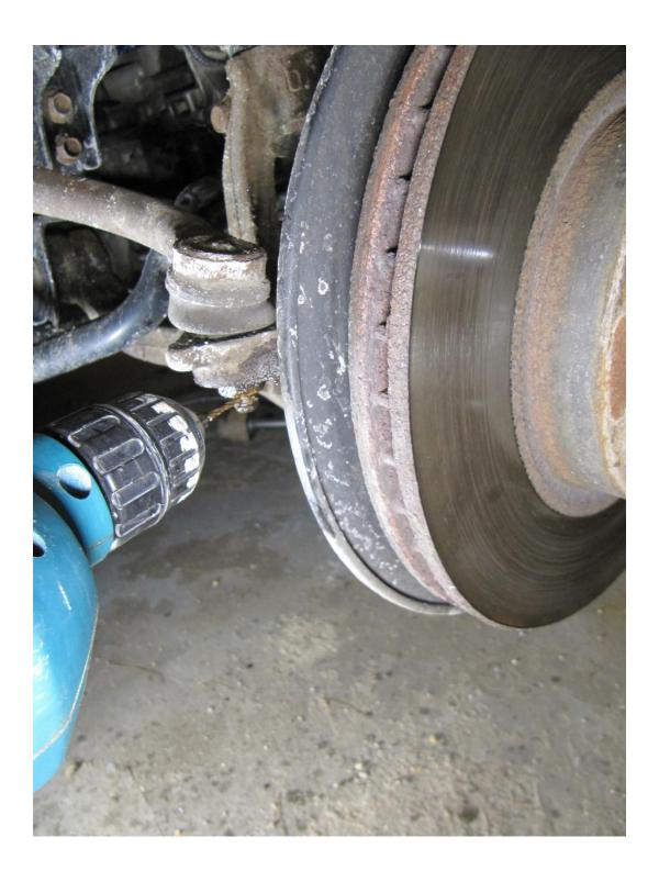
Loosen the tie rod end nut, but don't take the nut off completely yet:
