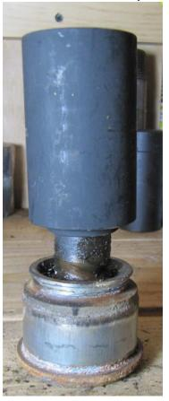
And the receiver cup isn't large enough to fit the base of the ball joint:
