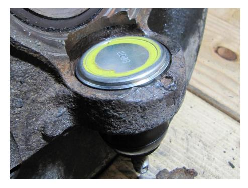
And notice that there is NO place for a snap ring on the bottom (No snap ring was present on the original factory ball joint, and no snap ring is needed for the replacement OEM ball joint. I believe some aftermarket ball joints do require a snap ring though):
