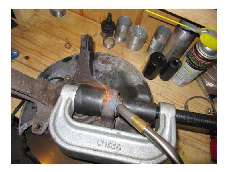
Then I used a half-inch ratchet and cheater bar to drive out the ball joint while holding the end of the knuckle in a bench vise. It wasn't too tough, but heating definitely made a big difference.
