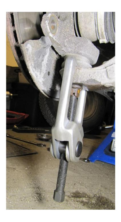
The knuckle should now be free to be pulled entirely out. Be careful to not pull the axle too far out in the process of removing the knuckle so you don't accidentally separate the internal CV joints.
