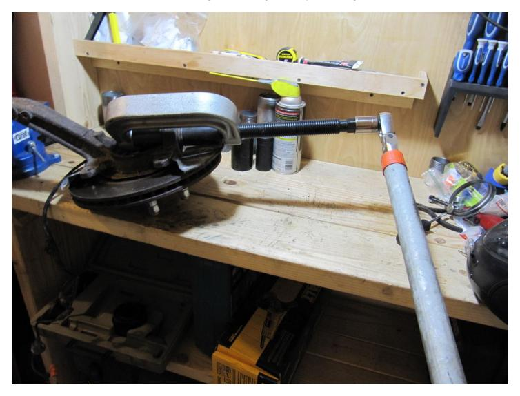
Once the ball joint was out, I cleaned up the ball joint seating surface (arrow) with the wire wheel:
