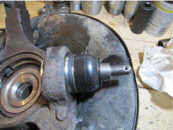
This image shows the ball joint fully seated in the knuckle:
