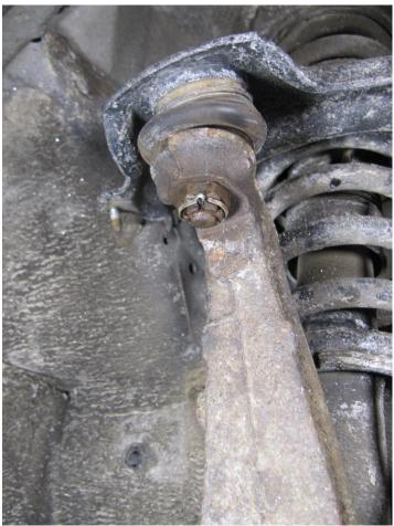
Install the lower ball joint nut and torque to 78Nm. Install a new cotter pin:
